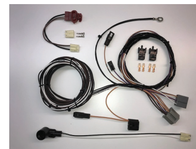
p/n 510484 80-86 Optional Dual Fuel Tank Harness
